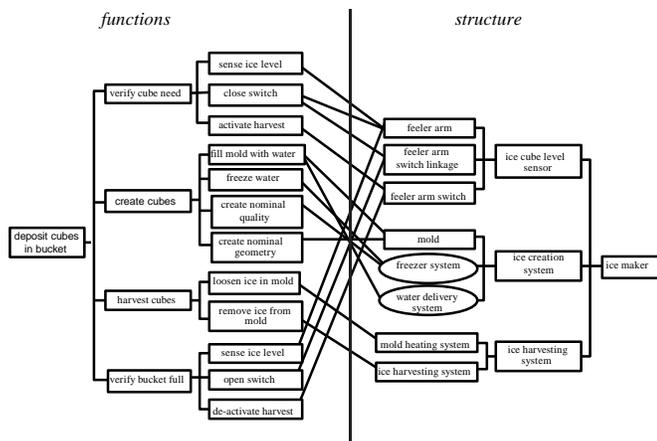
**Figure 2: Function-Structure Mapping**
