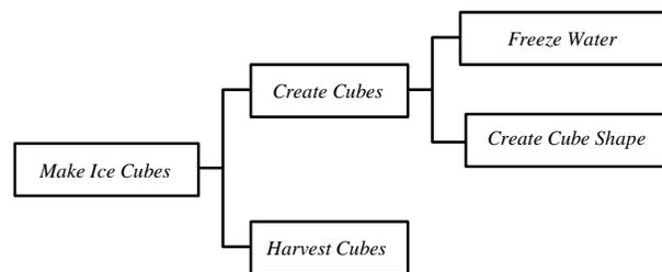
**Figure 1: Function Block Diagram for Ice Maker**
