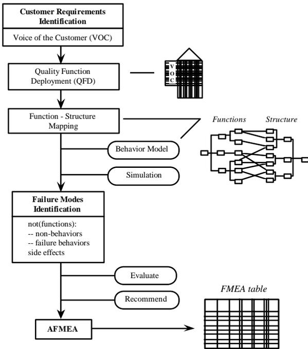
**Figure 4: Flow Chart of the AFMEA Process**
